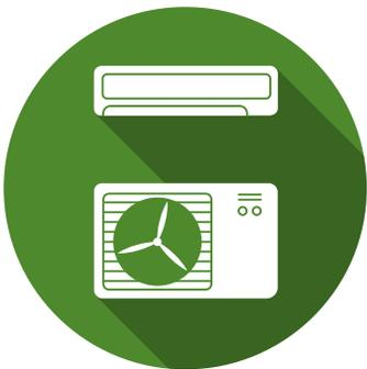
Air-source heat pumps extract heat from outside air that is then used for heating indoor spaces during the colder months. They can also extract heat from indoors and expel it outside to cool indoor spaces during the warmer months. Cold-climate air source heat pumps can replace your existing heating and cooling systems or provide supplemental temperature control in targeted areas of your home.
