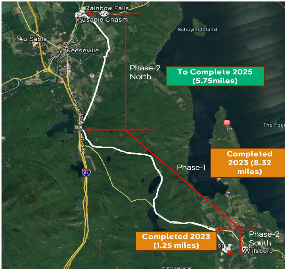
Figure 1: Proposed -15.32 miles of new Transmission Line 880 from Cabot Substation to Rainbow Substation. Phase I and Phase II South (total 9.57 miles) were completed in 2023. Phase II North from Structure 127 to Rainbow Substation (total 5.75) miles to complete in December 2025.
