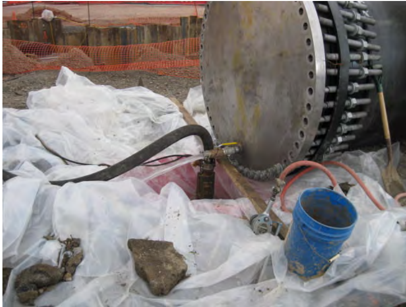
View of HDPE draining after leak test.
