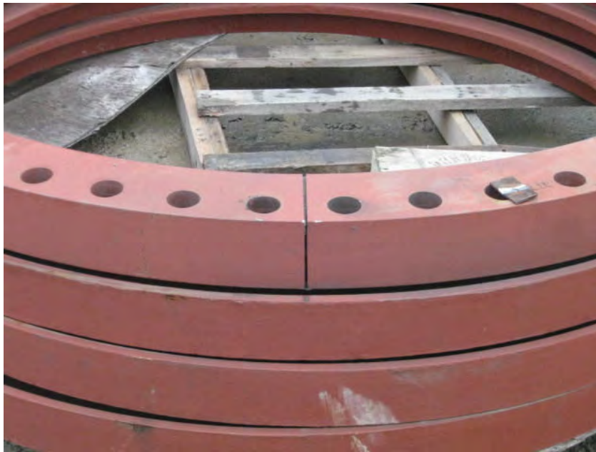
View of backer ring showing cut made by Tioga to fit ring over the HDPE pipe.
