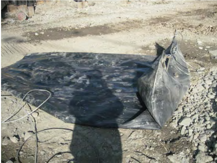
View of one of the inflatable pipe plugs used during the leak testing of the HDPE pipe.
